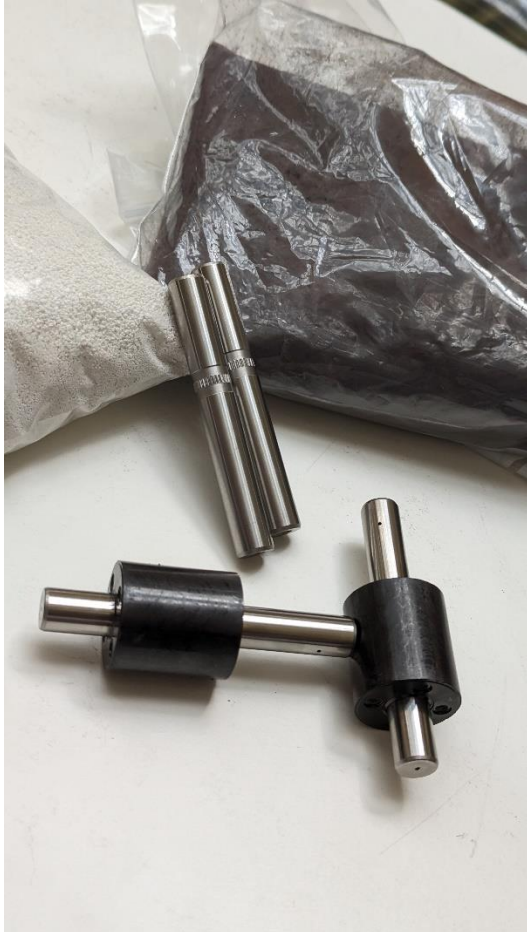
Rotor with PASSENGER's ferrite material directly molded onto the shaft
